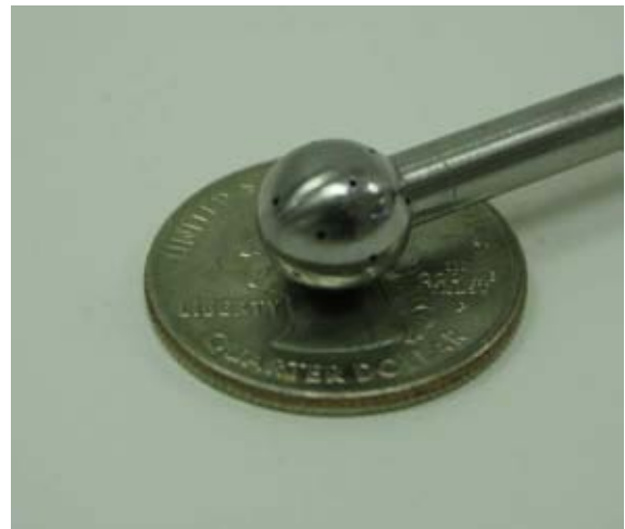
Figure 4: 9.53mm Omniprobe Tip
